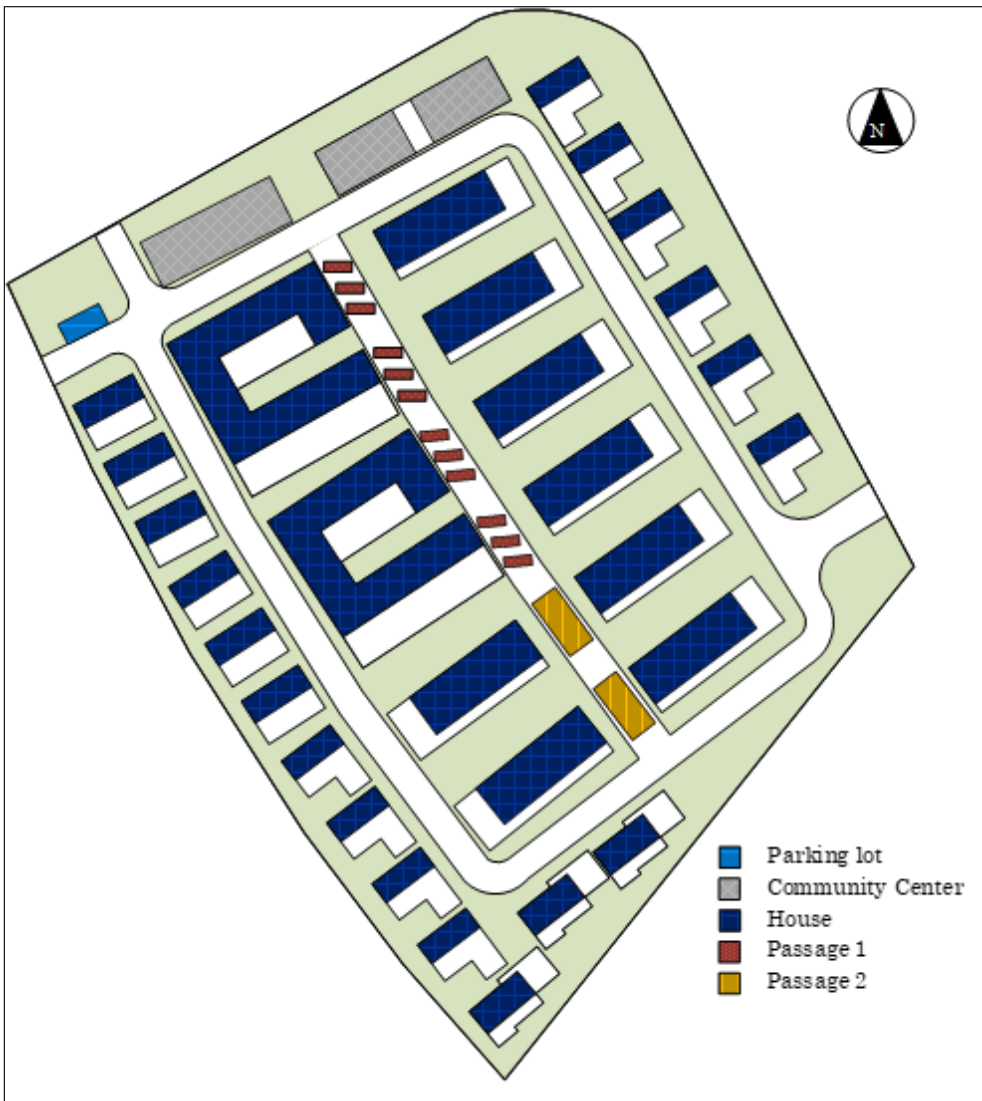
Figure 4. Target housing complex and arrangement of photovoltaic panels
